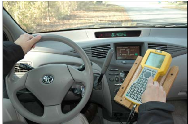
PICTURE 2 – Travel time data is collected using a GPS-equipped probe vehicle.
